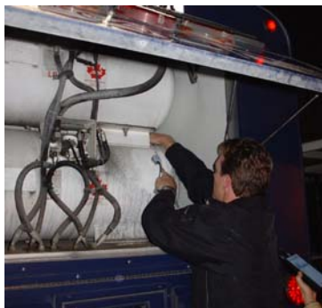
Picture 17: Measuring the Maximus™ Detected Liquid Level after Refueling
