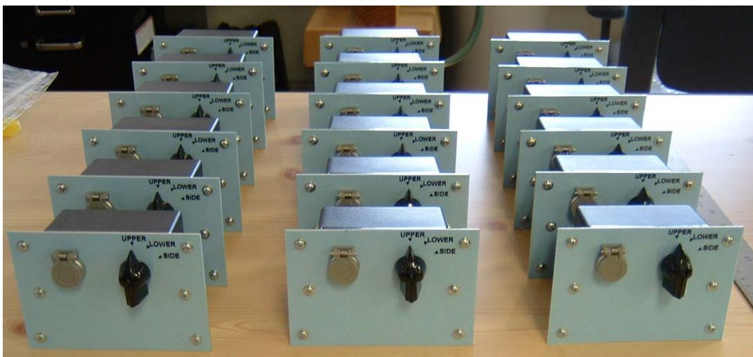
Picture 18: Junction Boxes with Quick-release Connector + 3-Position Switch
